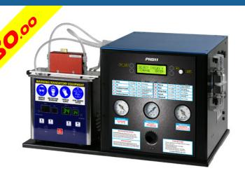
The Ultrasonic Cleaner Kit allows cleaning a large variety of inkjet print heads. It is equipped with a pump and an ultrasonic bath. It will work with any low-viscosity cleaning solution. The pump unit will run the solution through a print head, while the ultrasonic tank helps unclog the blocked nozzles by the action of high-frequency sound in the fluid.
